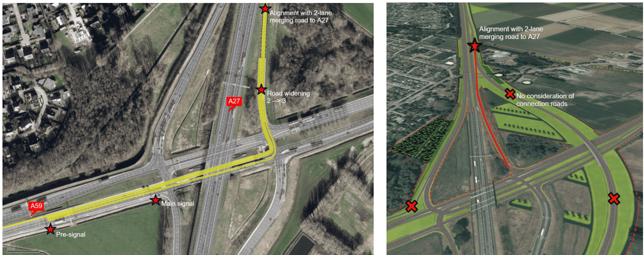
Figure 5.5. – Road Section That Facilitates a Pre-Signal System Size of 3 Lanes in Left-Turning Direction (left) and Alignment With Construction Design (right)
